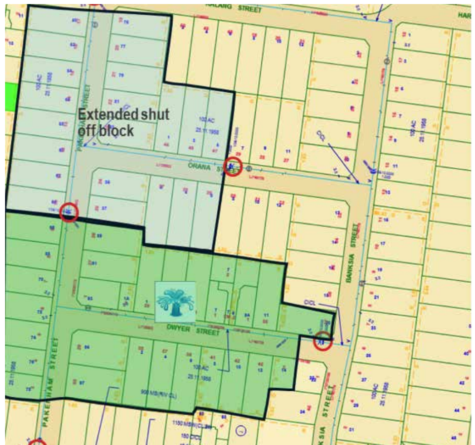
Figure 17: Customers impacted by a burst event
